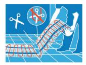
The heating mat installation starts from the wall and is directed towards the opposite wall. The mat can be turned around by cutting the net of the heating mat (please, do not cut the cable). The instalment of the heating mat has to be continued till it covers the entire area.
