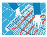
The floor heating mat should be installed onto clean surface.
